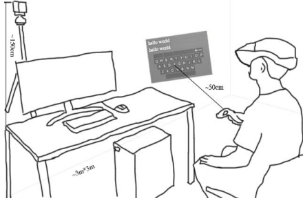
Figure 5: This figure shows the experimental setup. The HTC Vive optical trackers were placed at 1.5m high and had a tracking space with 3 \times 3m^2 . The keyboard is roughly 0.5m away from the participant which is recommended by the developers of the Meta 2.
